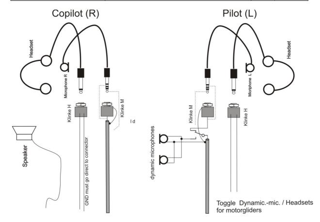
Because the 8V supply voltage is switched off when dynamic microphones are used during glider flight the second (copilot) headset microphone is disabled.
