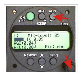
By pressing the DUAL button repeatedly L, R and AUTO can be selected. L (R) means left (right) microphone input channel. The AUTO function is explained later.
