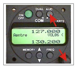
Any action in the Audio Menu requires the pointer (<) to be next to the Audio menu window (see picture). When the pointer is next to the Standby frequency window, the pointer can be repositioned by pressing the AUD button once.
