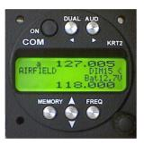
Display lighting current drain at maximum brightness is only 10mA. Maximum brightness is glare free even in darkness and can be used continuously. Indication of battery voltage (VDC).
